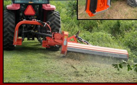
The flail head on the TLA series can all be quickly adjusted in and out with the tractor hydraulics. It can be adjusted from vertical (to mow tree lines and hedges), all the way down to 60 degrees below horizontal (to mow ditch banks).
