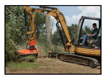
The image to the left shows a Lipa TLBE-100 on a CAT 304CR mini excavator. This 9800 lb machine had a maximum auxiliary flow of 18.5 gallon per minute. The TLBE-100 only requires 15-16 gallons per minute, so we added an optional flow regulating block to regulate the flow down. By adjusting the flow, the rotor speed can be set to around 2300 RPM, to optimize the mower performance and maximize flail life.
