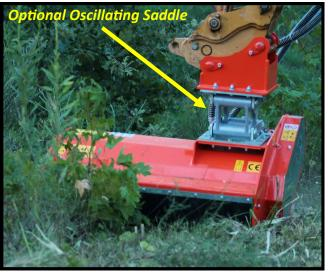
The Lipa TLBE-100 shown in the image left is fitted with the optional oscillating saddle. This is an excellent option if mowing a lot of uneven ground. This saddle allows the mower to follow the ground much better with a lot less operator adjustment. The TLBE mowers do not come with hydraulic hoses, these can be supplied by Needham Ag, or sourced locally.
