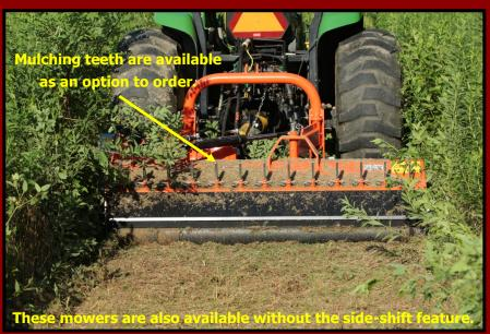
The TLS Flail Mower is perfect for mowing and shredding dense grass, brush and small trees up to around 3" in diameter. They cut/mulch finer than rotary cutters and provide a more even finish. This mower also features a heavy duty rear roller and has optional side skids.
