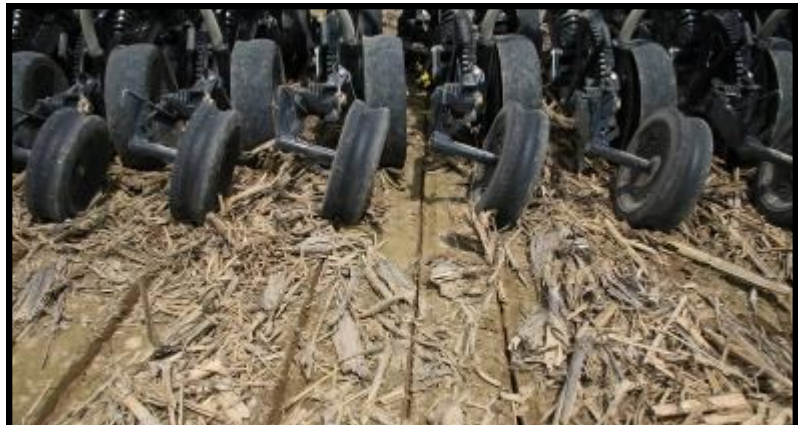
Factory 4 x 12 closing wheels on a Case-IH 500, with maximum closing wheel down-pressure. These wheels do a poor job closing, especially in moist no-till conditions.
