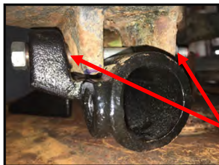
Seed Boot Bushings Pull Tight Against The Arm And The Boot Pivots On The Bushings.
