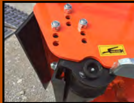
TLBE-90 with Deere wedge-lock coupler on a 35G. Optional hydraulic hoses and oscillating carriage shown
