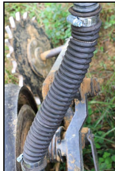
Cross-section of a stretched seed tube, showing the folds.
