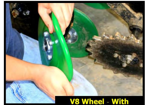
V8 Wheel - With Flexible Urethane Tire
