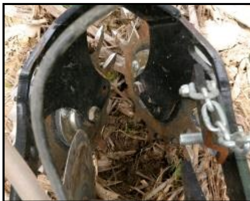
Martin row cleaners working in 200 bu/ac corn residue. Notice how they clear a narrow path for the UMO fertilizer opener.
