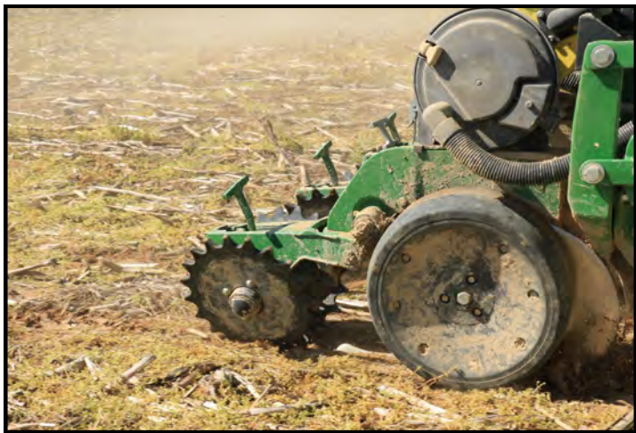
Here the same DB60 as shown above, is operating in a field which was vertical tilled the previous fall, with no spring tillage. Minimal down pressure was needed to close the seed slot within these conditions.
