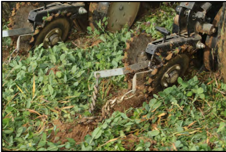
The Needham Ag Poly 20 Point Wheels being used on a Kinze 3000 series planter in pea and crimson clover cover crop. Minimal down pressure was required to close the seed slot and maximum performance comes when the closing wheel arm is level to slightly higher at the rear.
