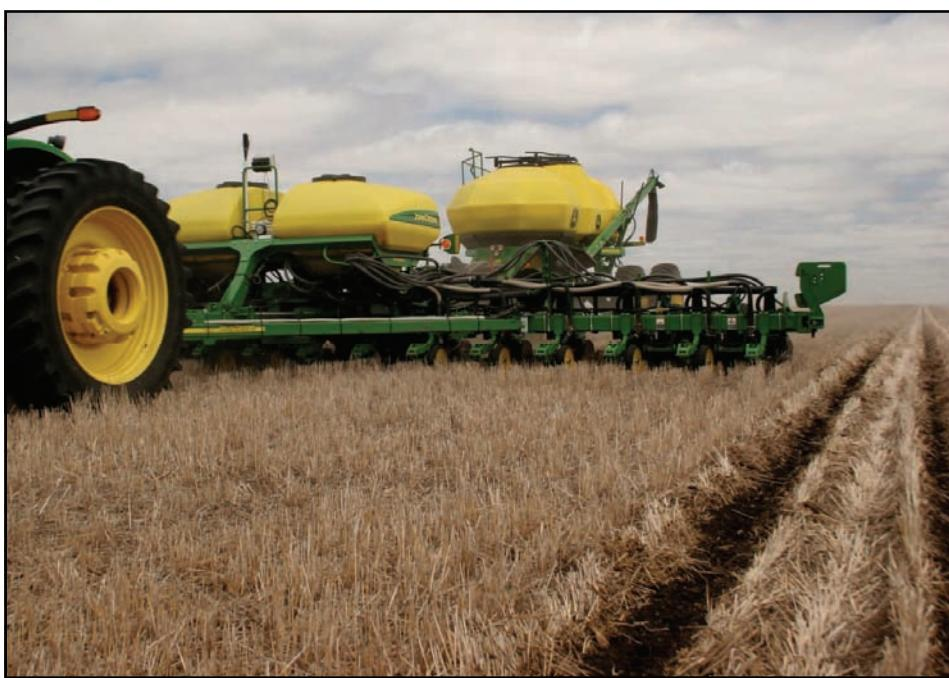
The image above illustrates a grower who plants with a 16 row John Deere 1770 planter and pulls a John Deere 3 hopper commodity cart behind it. This commodity cart configuration offers huge flexibility to deliver N + P + K in a consistent band alongside the row. If growers want to use variable rate fertilizer, this highly efficient system adapts extremely well.
