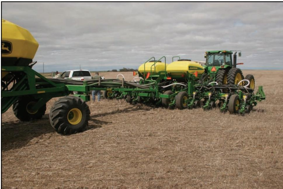
The image above illustrates how a commodity cart was coupled to a 12 row John Deere 1770 planter. While most commodity carts are now available to match 30" rows and most planters can be equipped with frame or unit mounted fertilizer openers, the hoses, manifolds and dry boots. These will probably need to be fabricated at the dealership or on the farm, because they are not yet currently available as a bundle from the manufacturer.
