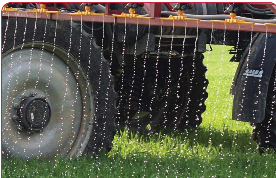
Liquid nitrogen can be easier to apply with farmer-owned or custom equipment with stream bars that minimize leaf injury and maximize uniformity.
