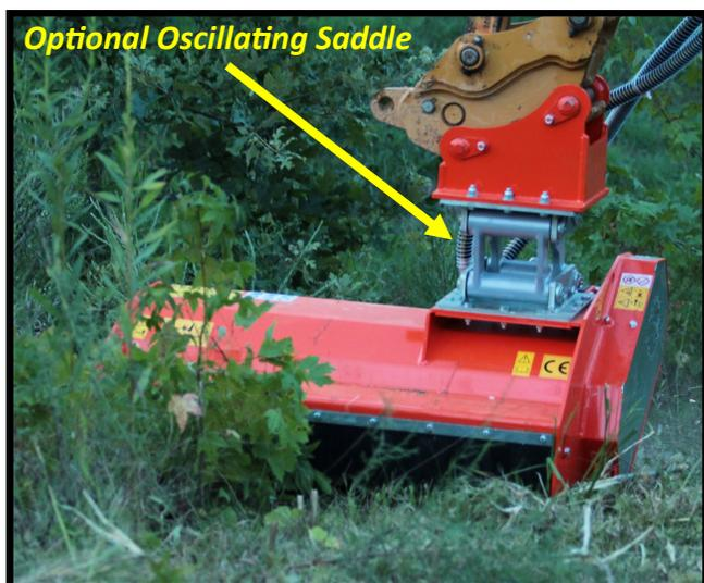
The Lipa TLBE-100 shown in the image left is fitted with the optional oscillating saddle. This is an excellent option if mowing a lot of uneven ground. This saddle allows the mower to follow the ground much better with a lot less operator adjustment. The TLBE mowers do not come with hydraulic hoses, these can be supplied by Needham Ag, or sourced locally.
