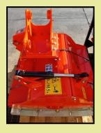
The standard option is a manual adjust front door, but if you have a mini excavator with a 2nd set of auxiliary lines, then you can order the TLBE-SF mower with a hydraulic cylinder on the front door. This allows you to raise and lower it like you would the thumb, to be able to cut the top out of trees, then lower the front door to control flying debris.
