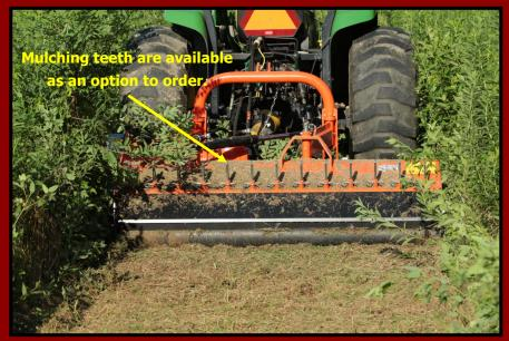
The TLC Heavy Duty Flail Mower is perfect for mowing and shredding dense grass, brush and small trees up to around 3" in diameter.
