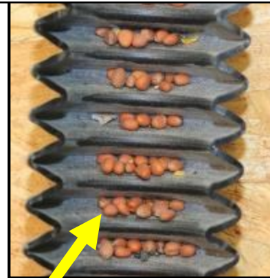
Radish seeds hanging in a factory seed tube angled at only 30 degrees from vertical.
