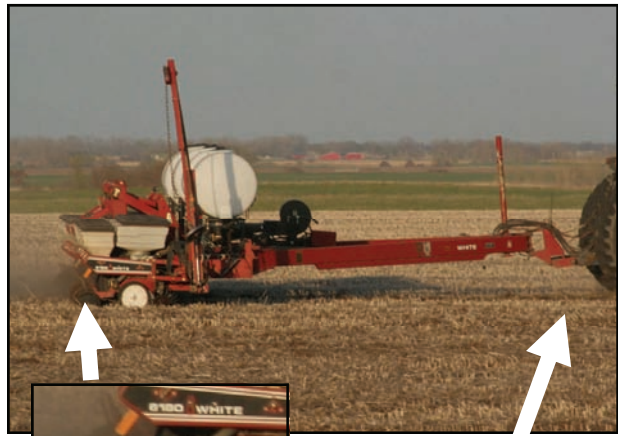
As the drawbar is raised at the tongue end, the closing wheel arms will raise at the back.
