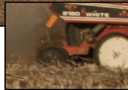
As the drawbar is raised at the tongue end, the closing wheel arms will raise at the back.
