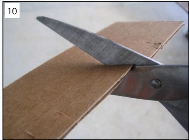
Image 9 (above) illustrates a pair of scissors with a low included angle, trying to cut through cardboard. The amount of force required to cut into the cardboard, even with sharp scissors is almost beyond what is humanly possible at this angle.
