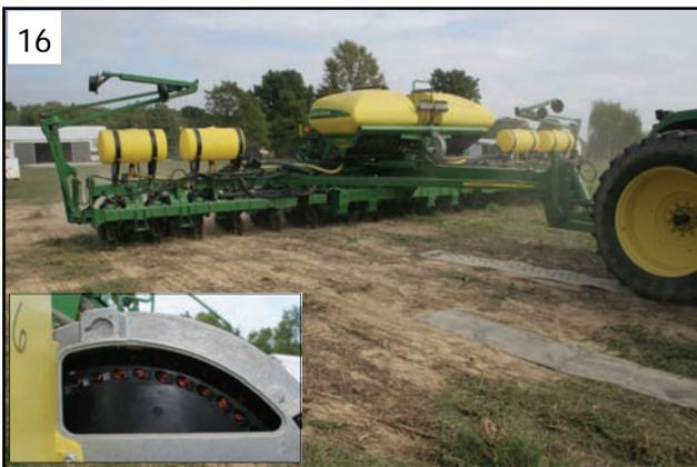
Driving a John Deere 1790 over rubber belts to determine the wheat seed population. Picking up a consistent number of seeds with a milo plate (inset image above) became a challenge, especially within no-till conditions and 5-6 mph forward speeds (even with higher vacuum).
